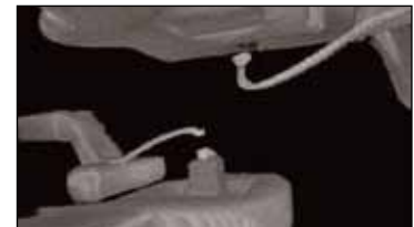
Damaged wirebond in IC
